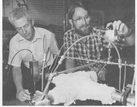
NEW LASER-LIKE LIGHT SOURCE developed by Arlee Smith (1124, left) and Joe Alford (1128) is nearly a thousand times more efficient than previous light sources operating in the ultraviolet portion of the electomagnetic spectrum. Here, the two are working with a "heat-pipe oven." Heated in the middle and cooled on the ends, the criss-crossed pipes provide the mercury vapor the new light source needs.
